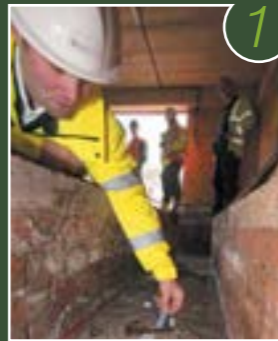
Step One Test the water for contaminants with the oil detection strips
